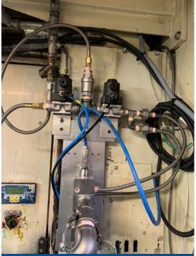
**FIGURE 7.** Viscometer installed using a flow adapter, showing the control valves for precise dosing of solvent to regulate ink viscosity.
