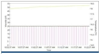
**FIGURE 9a.** Temperature-compensated viscosity (black. 25cP) and temperature (green, ~18° C) vs. time, coarse vertical scale
