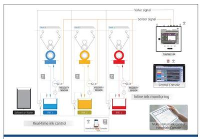
**FIGURE 6.** Real-time ink control is achieved through in-line ink monitoring facilitated by placement of viscosity sensors at each print deck. They connect and transmit data to a central multi-station and single-station handheld consoles.
